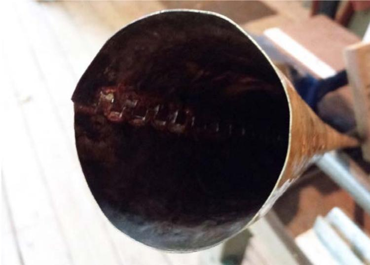
The curved piece of flat brass is annealed, then soldered to form the garland which will slide over the bell. Decorative points are carefully cut into the garland, and it can be engraved by hand as well.
