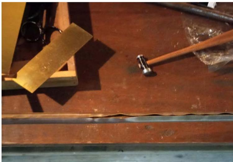
Three lengths of tubing, annealed, formed, and soldered, each of which started out as flat pieces of brass. The shortest tube is being polished, as the others will be in turn. 🤏
