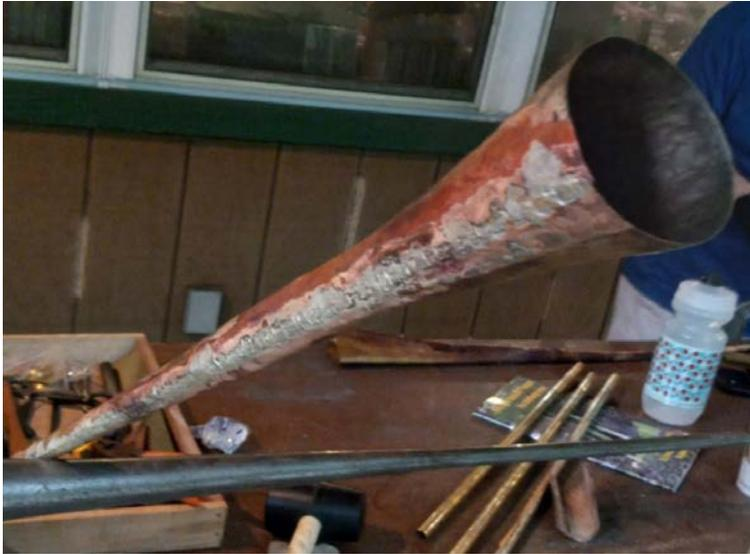
One of the straight tubes is now cut into 2 pieces, which are filled with a hard resin and left overnight. In the morning, they are bent by hand around a wooden form to create the 2 bows, one at either end of the finished trumpet. After bending, the bows will be cut to their finished length, the hand-polished.
