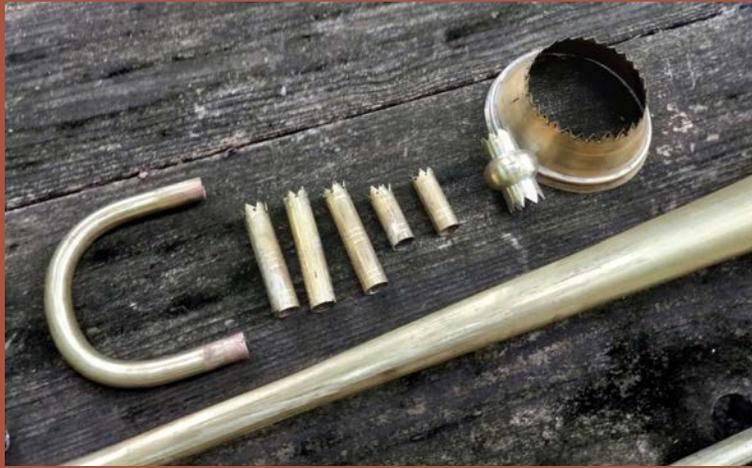
Pretty soon all the pieces will be assembled into a finished product. The brass surface is hand-scraped with a special tool, then further polished with fine sandpaper and steel wool, to the maker's taste.
