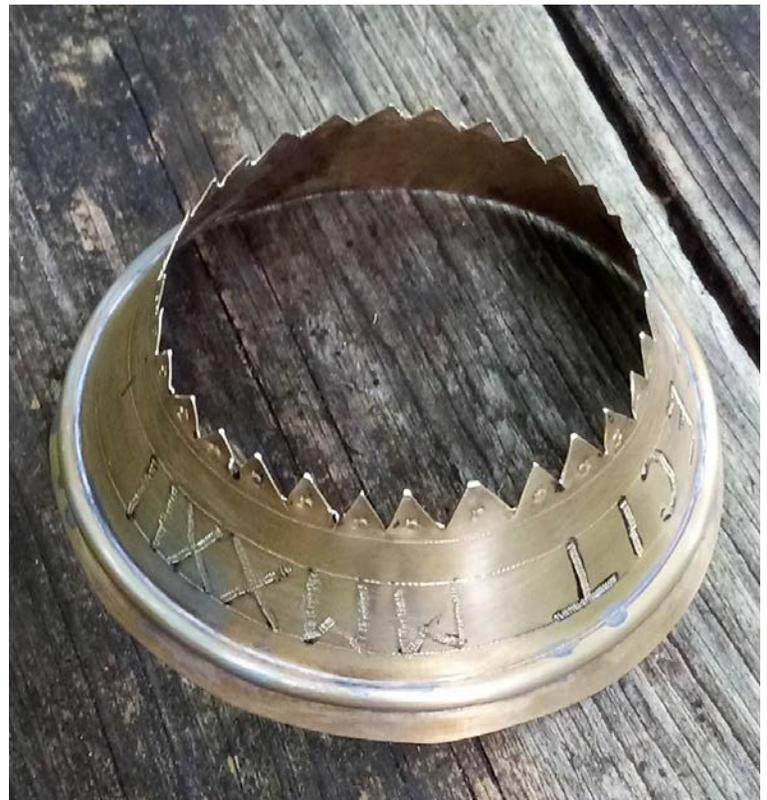
Another tube is cut into 5 pieces, which become the ferrules used to strengthen all the joints where the tubes come together. These are decorated as well with a star pattern. measured and cut by hand. The decorative ball which fits over the bell is assembled, soldered, decorations cut and then polished.
