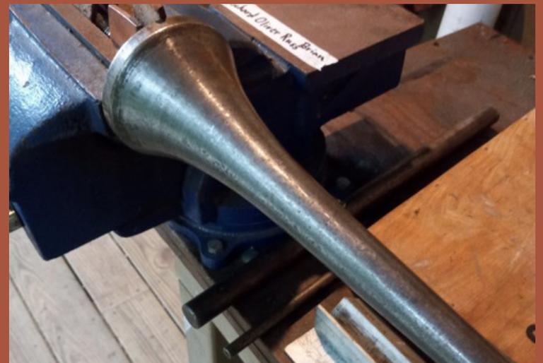
After hours of working on the anvil and mandril, with heating in between, the bell is nearly formed.
