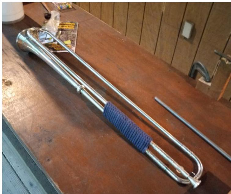
Four sheets of brass, and a curved piece (destined to become the bell garland) are 90% of the materials used to make an entire trumpet!
