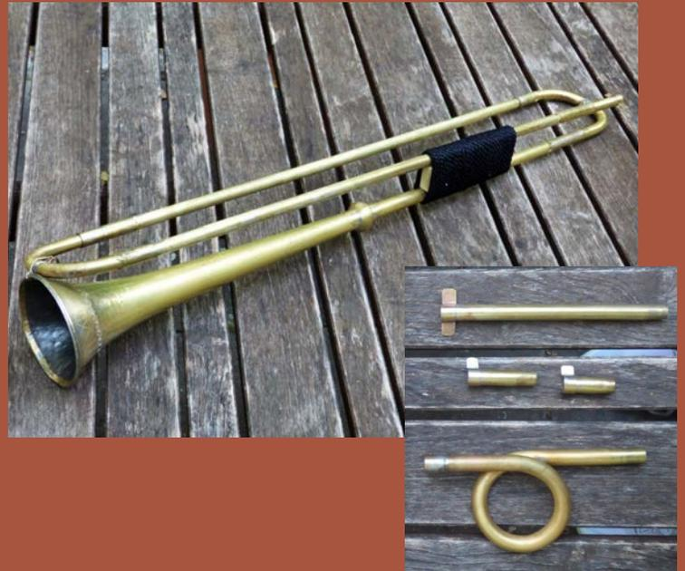
We cut additional tubing into several lengths, to fashion tuning bits. This allows the trumpet to play in different keys (D 415, C 440 and C 415), while the smallest ones also allow for some fine tuning. The pigtail (putting the horn in C 415) was made for each of us by the instructors, as this fine work was likely a bit beyond our reach! 🐷
