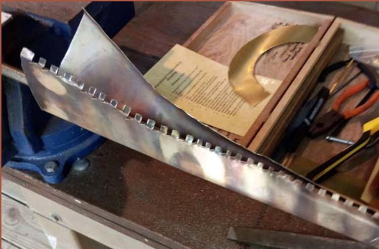
Using a piece of wire to hold the metal together as the teeth are hammered into the opposite side.
