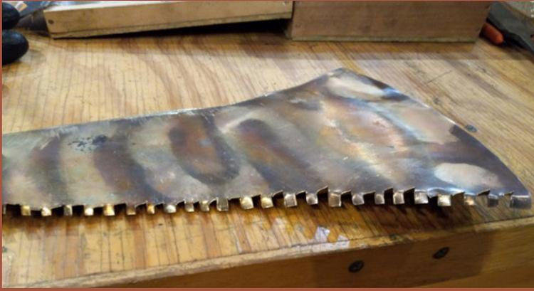
Starting to bend the sheet around the mandrel, to get the teeth to meet the other side and form a joint which can be hammered smooth, then soldered.
