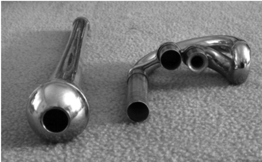
Figure 19: Isaac Fiske echo attachment. Note the constriction at the upstream end. (Photo: Robert Pyle)
